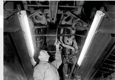
B.R. Bailey's first Craft Lite or known at the time as a "Hoist Lite" was used on service station hoists and allowed the workers to work easily with both hands.
