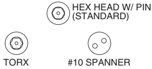
TAMPER RESISTANT SCREW HEADS OPTION SUFFIX- T3
