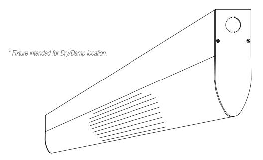
**Cleaning Instructions:** Wipe luminaire with a soft cloth slightly dampened with warm, soapy water. On stainless steel units, tightly adhering deposits may be removed by using a stainless steel polishing powder. Never use steel wool or steel brushes on stainless steel. Always rub in the direction of the polish lines.
