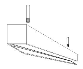
**Cleaning Instructions:** Wipe luminaire with a soft cloth slightly dampened with warm, soapy water. On stainless steel units, tightly adhering deposits may be removed by using a stainless steel polishing powder. Never use steel wool or steel brushes on stainless steel. Always rub in the direction of the polish lines.
