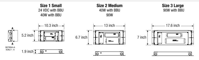
BBUX — Battery Backup & LED Driver Remote (Outdoor), IP67, IK10, NEMA 4X, -20 to 55 °C (-4 to 131 °F), 30 feet Maximum Distance with 12AWG (with UNV Option Only)
